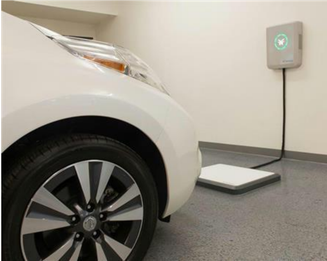
Figure 1. Wireless power transfer system of an EV and PHEV.
