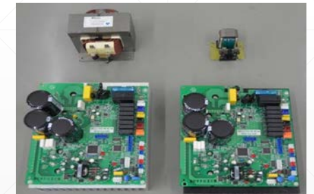
SiC can reduce coil size
