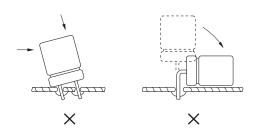
The main chemical solution of the electrolyte and the separator paper used in the capacitors are combustible. The electrolyte is conductive. When it comes in contact with the PC board, there is a possibility of pattern corrosion or short circuit between the circuit pattern which could in result smoking or catching fire. Do not locate any circuit pattern beneath the capacitor end seal.
