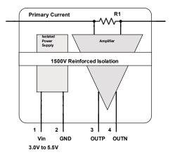
Amplified Analog Output and Reinforced Isolation
