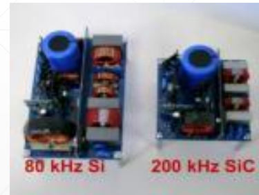
SiC solution for high frequencies
