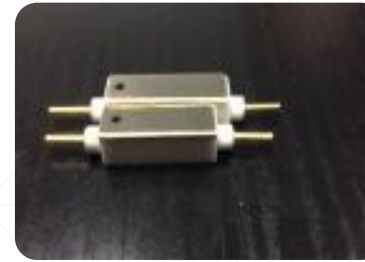
T_a=215^{\circ}\text{C} 7000V1A and 9000V1A diodes
