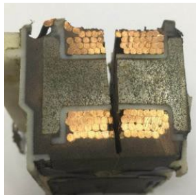
potting voids inspection
