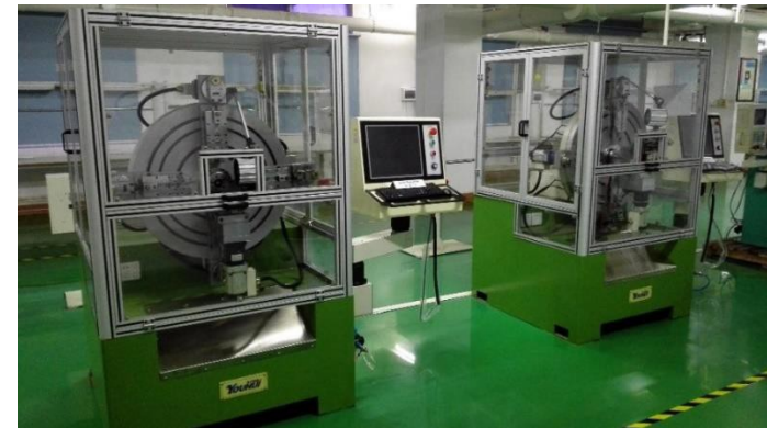
Helical Flat Wire Coils Winding
