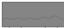
Severely crack: not acceptable. More obvious cracks extended from side to side.
