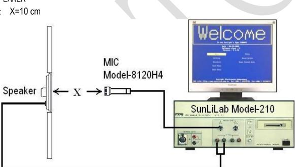
Standard Baffle Recommended In IEC 268-5 Where (W) 1350mm x (H) 1650mm
